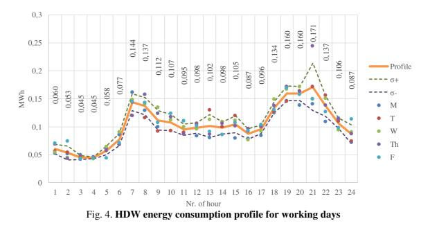
Regarding this, in further calculations to create a HDW consumption profile two separate cases were considered – working and non-working days. HDW consumption profiles were created using average data collected in Table 2, also standard deviation values were calculated and plotted. Fig. 4 and Fig. 5 show the HDW energy consumption profile for working and non-working days and the calculated values.
