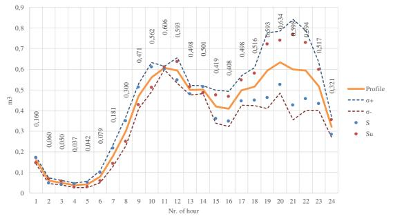
Fig. 7. HDW volume consumption profile for non-working days
