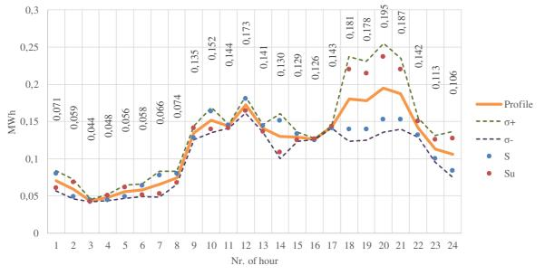
Fig. 5. HDW energy consumption profile for non-working days
