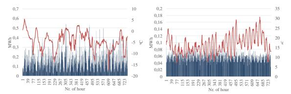
Fig. 1. Combined HDW energy consumption of January and July and outdoor temperature
