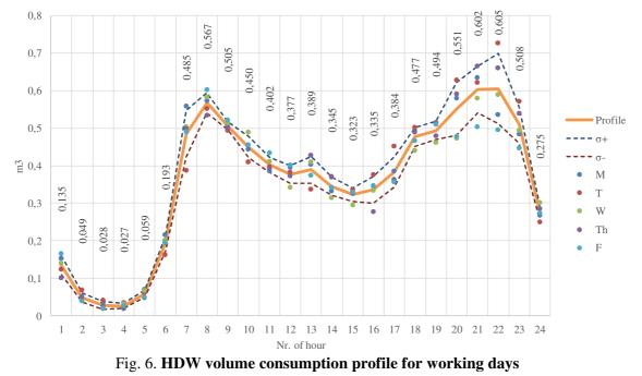
Similarly, profiles were created for the HWD volume consumption, as seen in Fig. 6 and Fig. 7. Spikes and drops are higher in these profiles, since in night hours consumption is close to  $0m^3$ . Similarly as with energy, also volume spikes during non-working days are longer and continue during day hours compared to working days, when only morning and evening spikes are dramatical.
